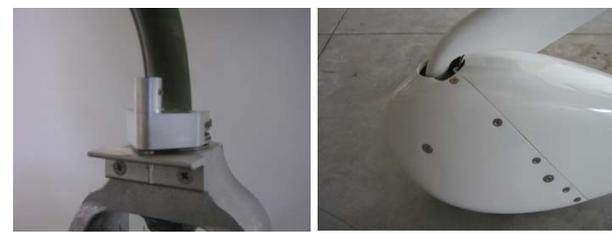
The Mishler Noselock System is an easily installed solution to help prevent nosewheel shimmies upon landing. The system effectively captivates the castoring action of the nosewheel during takeoff by means of a pin and barrel assembly. The pin and barrel are attached to the upper flange of the Velocity nose strut and, through a push-pull cable, the pin can be engaged in a piece of aluminum angle attached to the nose fork, which effectively limits the rotation of the fork.
