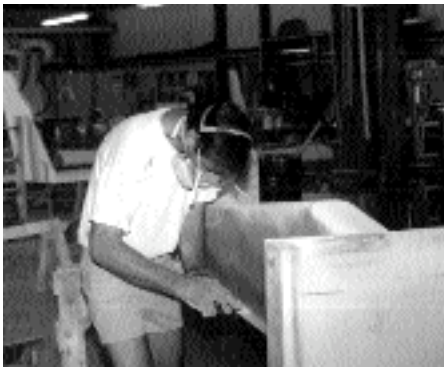
John Harvey constructing the new Elite center console mold
